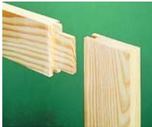
In the frame and raised panel article in issue No. 140, we showed how to build a stub tenon and groove door. This is a quick, easy-to-build frame if you've got relatively small doors, like those on the bookcase.
